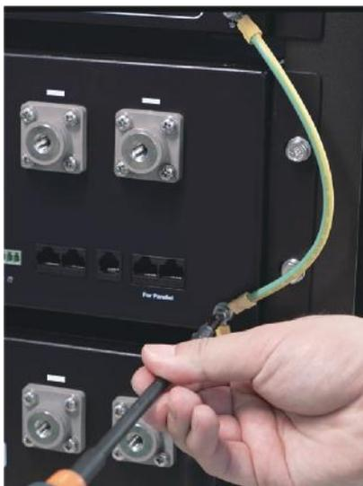
② Use the 5AWG terminal 200mm battery parallel wires included in the packaging to connect the batteries in parallel.
