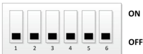
By setting the address through the dip switch on the BMS to distinguish different PACKs, it is necessary to avoid setting the address to be the same. The definition of the BMS dip switch refers to the table below, and the system supports a maximum of 32 parallel machines.
